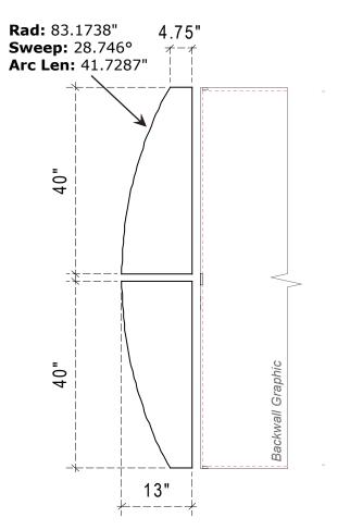
**NOTE:** These dimensions are for graphic layout purposes. Graphic needs to be cut and test fitted to Sacagawea frame.
