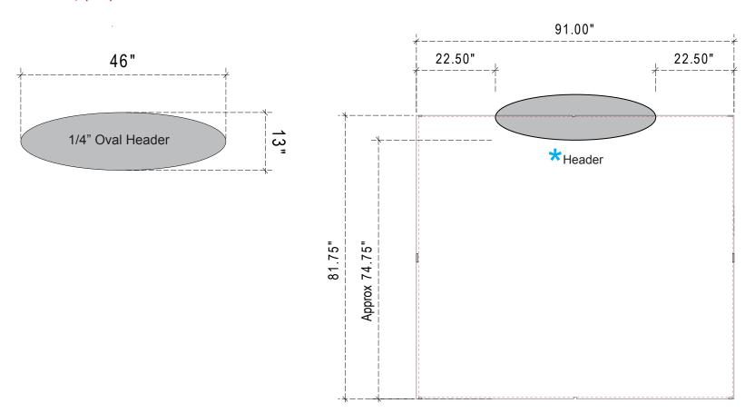
**NOTE:** When using headers with the Sacagawea unit a portion of the graphic will be covered. Please design graphic layout according to desired header shape and location.
